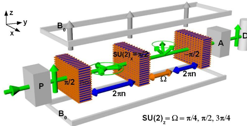
Intensity:  $I = |\langle +z | \hat{U}_{\text{out}}^{-\pi/2} \hat{U}_{L'}^{2n\pi-\eta} \hat{U}_0(\xi, \delta, \zeta) \hat{U}_L^\eta \hat{U}_{\text{in}}^{\pi/2} | +z \rangle|^2$
