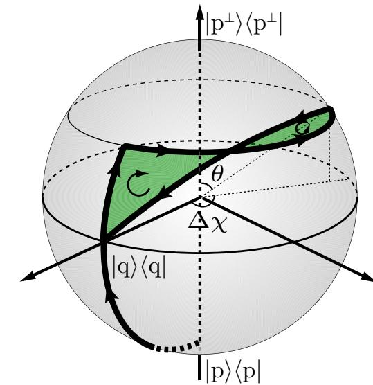
Superposition of Path 1 ( $|p\rangle$ ) & Path 2 ( $|p^\perp\rangle$  due to beamsplitter, absorber ( $T$ ) and phase shifter ( $\Delta\chi = \chi_2 - \chi_1$ ):
